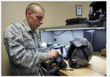
U.S. Air Force Airman 1st Class Sean Crowell, aircrew flight equipment technician with the 23d Operations Support Squadron, uses waxed thread to secure an oxygen mask to a pilot's helmet during the certifying and fitting of the Helmet Mounted Cueing System (HMCS) at Moody Air Force Base, Ga., Jan. 17, 2013.
