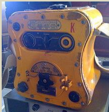
BC-778 "Gibson Girl" radio transmitter.
