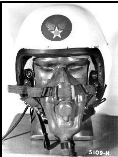
Figure 38: A front view of the prototype P-2 helmet with MS22001 mask.
