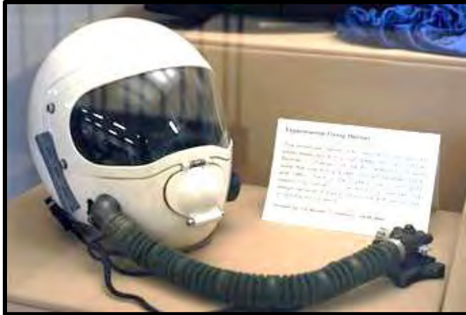
Figure 14: A rare HG-20/P precursor design, experimental wind-blast helmet (USAF) 1960, on display at the National Air & Space Museum.
