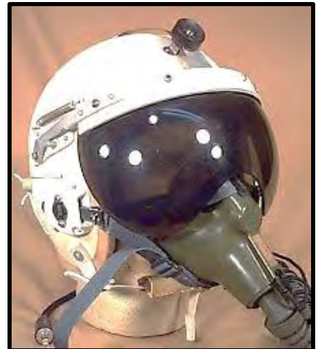
Figure 50: A P-4A helmet with Sierra Engineering Company bayonet receivers (MBU-5/P mask).
