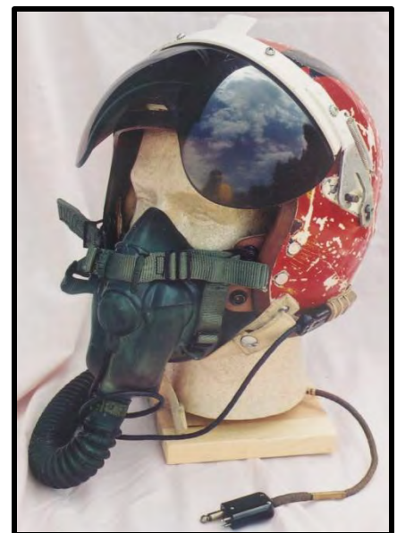
Figure 8: The USAF P-3, a P-1A with a visor added, 1953.
