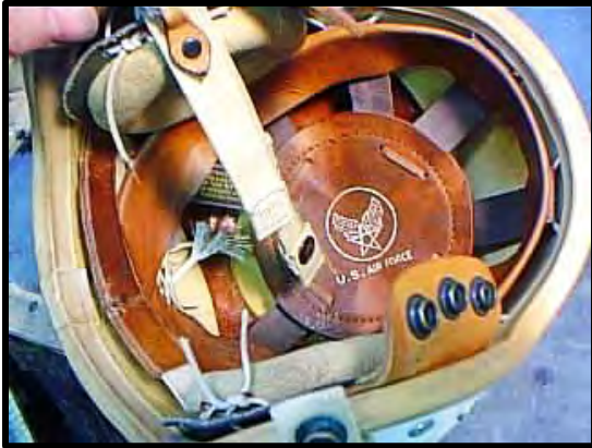
Figure 34: An interior view of a P-1A helmet; note the so-called "doughnut" earphone cushions (kapok filled chamois), characteristic of P-1 through P-3 helmets.
