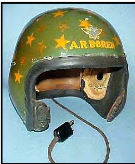
Figure 31: An original P-1 helmet that has not been upgraded to P-1A status; note earphone cushions have deteriorated and been removed.
